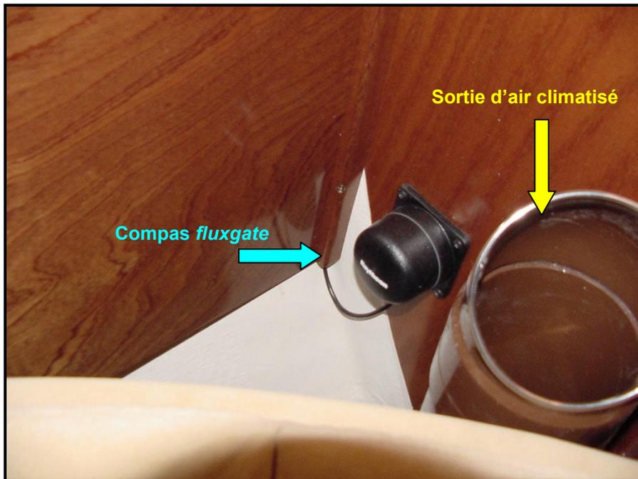
Figure 117 – Compas fluxgate
