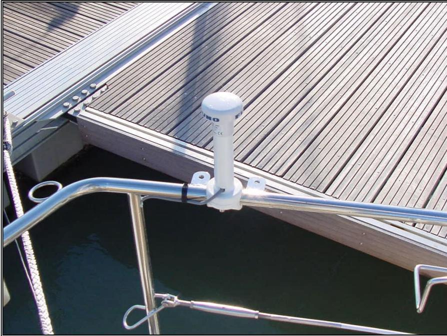
Figure 119 – Antenne GPS
